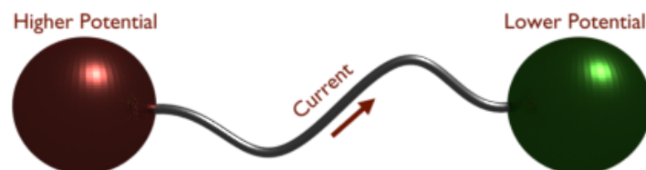
Fig.2.1 Current starts flowing from higher potential body to lower potential body
